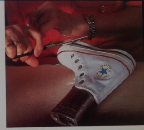
One of these parts is a strip of fabric called piping. The piping is coated with gum (a type of rubber, not something to chew). The piping is wrapped around the bottom of the sneaker, cut to fit, and then pressed in place with a roller.
