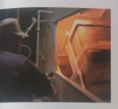
In a mill at the factory, rubber is mixed with clay, dyes, and chemicals to make it more durable and to give it color.
