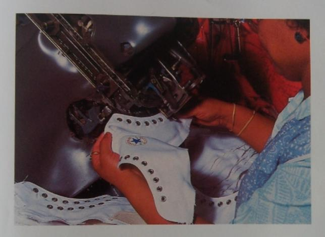
Eyelets with metal washers are then poked into the uppers. The washers add strength to the eyelets and keep the fabric from tearing when the laces are tied. The finished uppers are hung on hooks until they are ready for assembly. They are sorted according to their size, style, color, and whether they fit the left or right foot.
