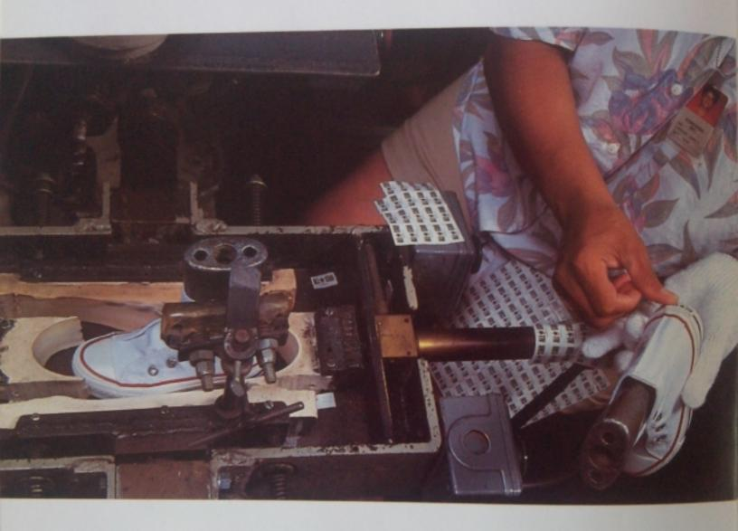
The brand label is glued to the heel of each finished sneaker. The sneaker is then placed in a hydraulic press, which squeezes the heel, toe, and sides together.
