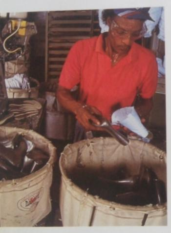
Each sneaker is assembled around a last, which is an aluminum mold shaped like a foot. Lasts are stored in baskets according to size, foot shape (left or right), and style.
