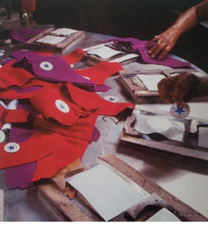
High-top sneakers have ankle patches with the brand name on the inner side of each upper. The patches are applied by hand. Then a rotating table carries the uppers to a sealing station. At the station the patches are firmly bonded to the fabric.
