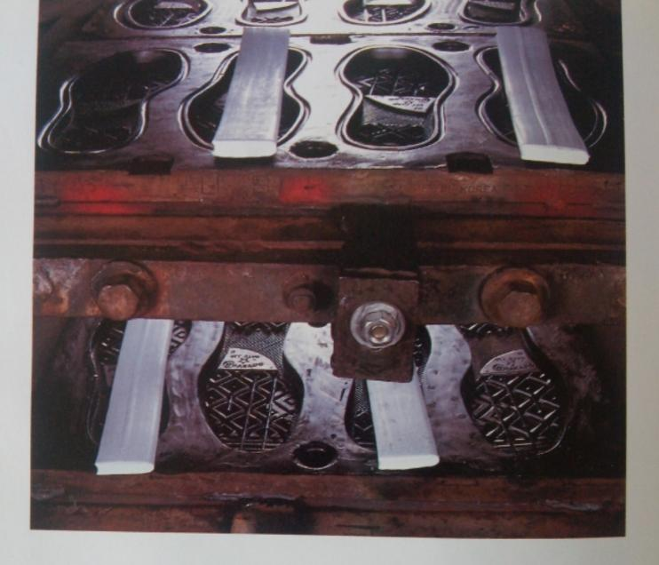
A slug is positioned on top of each mold. The curing press is closed and heated to 310° F. The heat causes the slug to compress and fill the mold. In less than three minutes the outsoles are completely baked.
