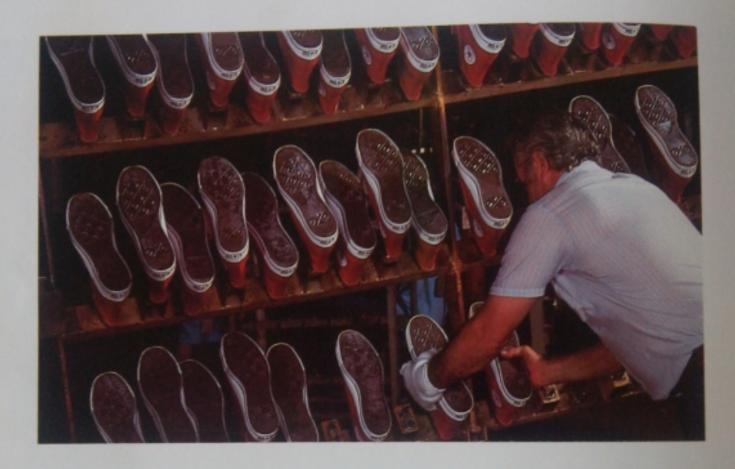
The sneakers are taken off the making line and placed on a rack. Each rack holds twenty-seven pairs. When twenty-one racks are filled, they are placed in a huge steel oven that is shaped like a tube. This oven is called a vulcanizer. It cures the sneakers by baking them for eighty-eight minutes at a temperature of 292° F. Curing helps give the sneakers strength and flexibility. When the time is up, the door opens automatically and the racks move out of the vulcanizer.
